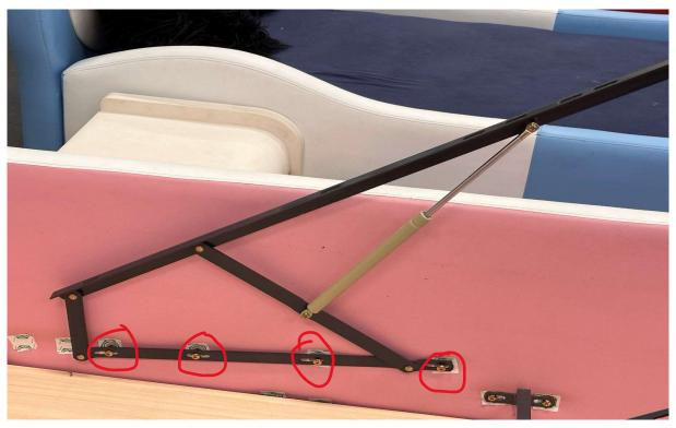
Finally, complete the assembly by attaching the mattress slats onto the gas lift assemblies. Ensure proper alignment by matching the holes on the mattress slats with those on the gas lift assemblies. Utilize the longer bolts provided for the three holes on each side and secure them with nuts.
